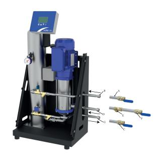
3. Connect the line (A) to the flexible outlet line (B) Connect the line (C) to the flexible outlet line (G)
