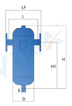
Body: Carbon Steel (Optional Stainless Steel) Interior: Carbon Steel (Optional Stainless Steel) **Connection:** Vertical – Threaded and Flanged **Diameter:** Threaded 1/2"-4" - Flanged DN15-DN300 Max. Operating Pressure: 16 Bar, 25 Bar, 40 Bar Max. Operating Temperature: 300 °C
